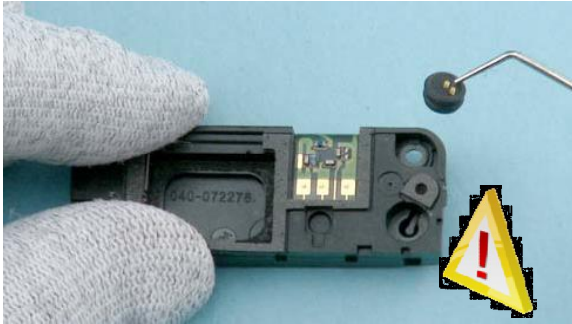
27) Use the dental tool to carefully lift up the MICROPHONE.
