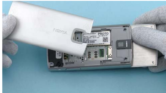
4) Remove the battery cover. If there is a battery inserted, remove it also.
