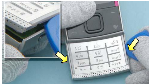
6) Use the SRT-6 to release the NUMERIC KEYMAT ASSY and the E-COVER ASSY.
